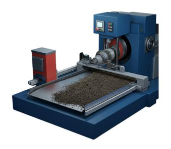
Adjust Rollers: Set roller pressure based on material thickness.
